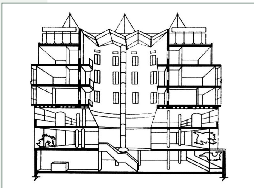
Cross section through the building, showing the centrally located atrium. Source: Murray O'Iaoire Architects
