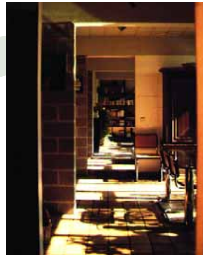
Willem House, Architect Jean Cosse. A tiled floor can be used to maintain the thermal link between the ground floor slab and a room's internal environment for more information see case study seven.
