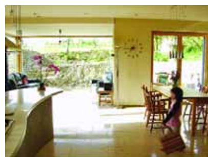
A ceramic tiled floor ensures that the transmitted solar radiation can be absorbed and stored in the building ground floor concrete slab. Source: MosArt
