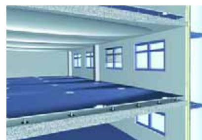
Profiled concrete soffit and floor void ventilation. Wave-form soffits are employed in the BRE building, while raised floors are used in the WIT library building; see case studies three and five. Source: The Concrete Centre
